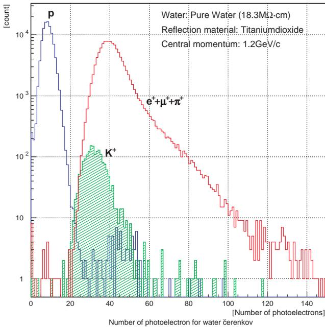
Fig. 4-2-5 Number of photoelectrons measured by the T494 pure-water Čerenkov counter. More than 99% of protons are separated without missing  $K^+$ s.
