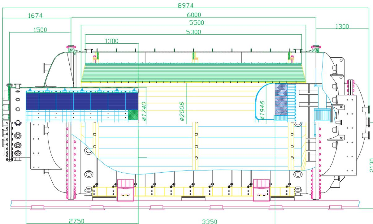
Fig. 4-2-2 Engineering design of the E391a detector to measure  $K_L^0 \rightarrow \pi^0 \nu \bar{\nu}$  rare-decays. Most of the detectors including a CsI calorimeter are placed inside one large vacuum vessel.
