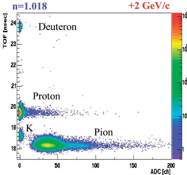
Fig. 4-2-6 Study of particle identification by a combination of aerogel counter and TOF for the PHENIX experiment (T496).
