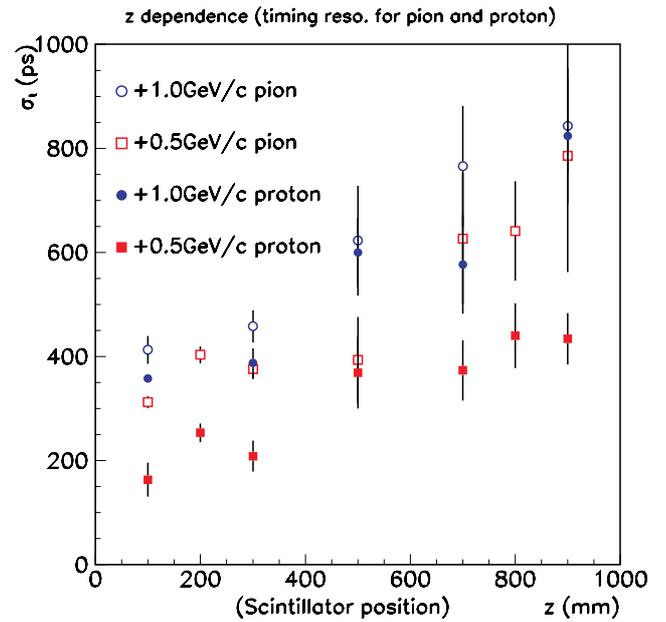
Fig. 4-2-7 TOF resolutions obtained by a fine-segmented TOF hodoscope (5 mm × 10 mm × 1,000 mm) made of fiber bundles read out by multi-anode PMTs (T502).
