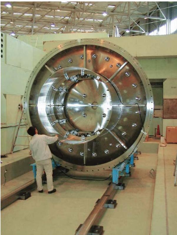
Fig. 4-2-3 Downstream section of the E391a vacuum vessel placed in the PS experimental hall.
