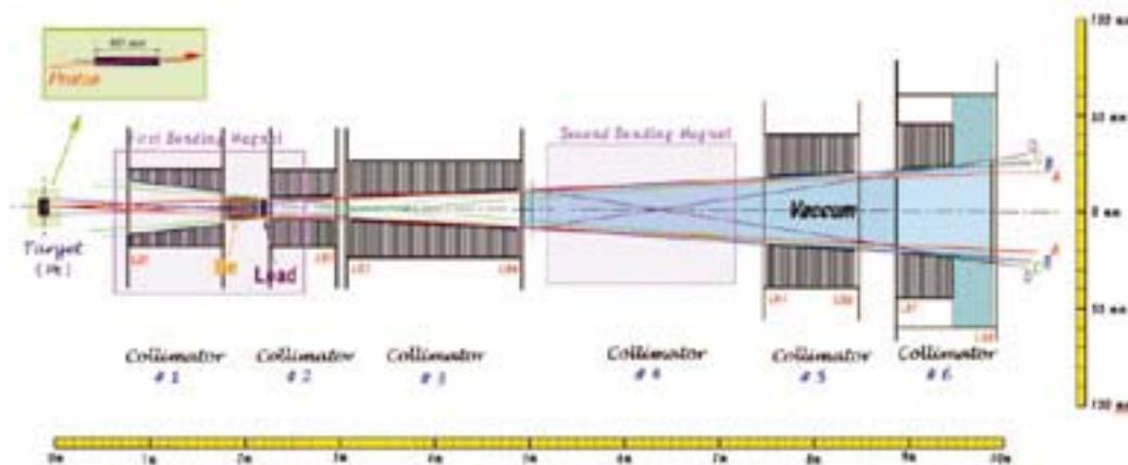
Fig. 4-2-3 New  $K^0$  beam line for Experiment E391a.
