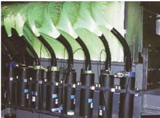
Fig. 4-2-5 Side view of a 1 m-long prototype of the barrel  $\gamma$  veto detector for Experiment E391a.
