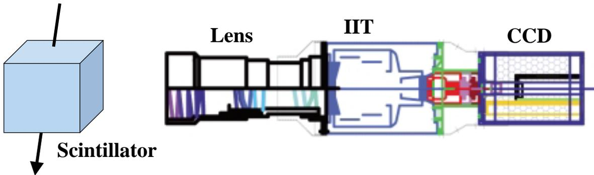
Fig. 4-2-7 New SCITIC (SCIntillating Track Image Camera) track detector developed by the E452 group.
