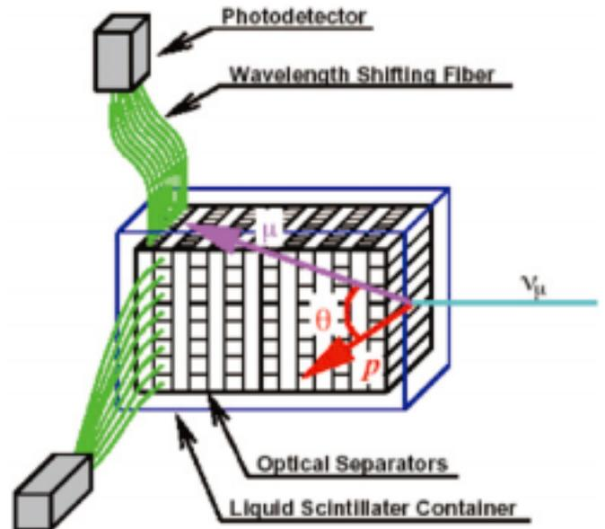
Fig. 4-2-9 Schematic view of the fine-segmented liquid scintillator detector with wave-length-shifting (WLS) fiber readout; one of the candidates for the neutrino detector in upgrading the near detector system of the K2K experiment.
