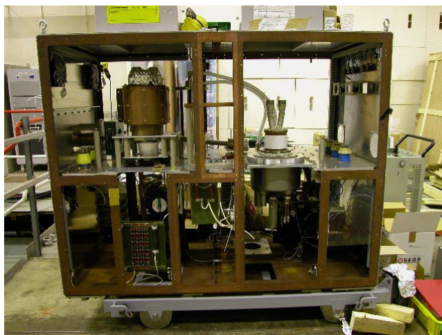
Photo 1: HPD with power tubes
