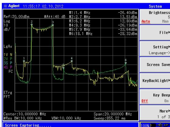
Fig. 5: Frequency spectra of the new digital MO (green) and the old one (yellow). Subharmonic peak locates at 1.4MHz (marker 1) and the 2RF spectrum ranges from 2.7 to 6.2MHz (between markers 2 and 3). The difference of amplitude between 1.4MHz and 2.7MHz components is -60dB for the new MO.
