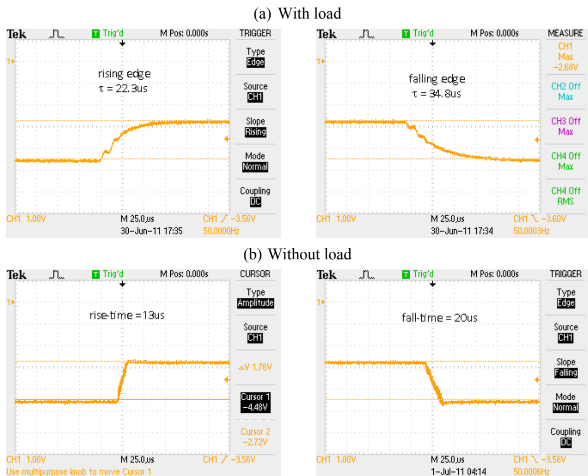
Fig. 7: Output voltage of the grid switcher (a) with and (b) without load.
