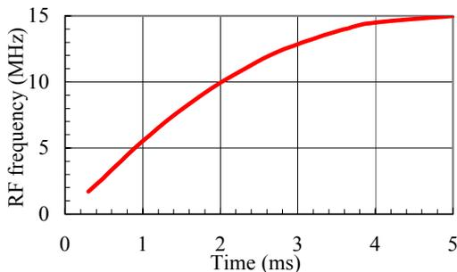
Figure 1: RF frequency as function of acceleration time.
