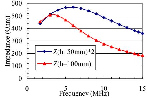
Figure 3: Cavity impedance. (upper curve, 4 cores loaded in 2 cavities; lower curve, 4 cores loaded in 1 cavity)
