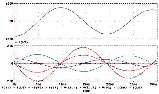
Figure 4: Current and voltage behaviors of the multi-mesh circuit. (a) Terminal voltage of each dipole, and (b) currents and voltages at the probe points in Fig.3.
