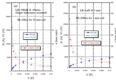
Figure 2: Estimations of capacitor, turn ratio of the matching transformer, primary current and capacitor voltage for exciting one dipole magnet up to the maximum field for (a) 10 turn coil and (b) 1 turn coil.
