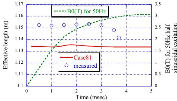
Figure 7: Measured and calculated (Case81) effective magnet length.
