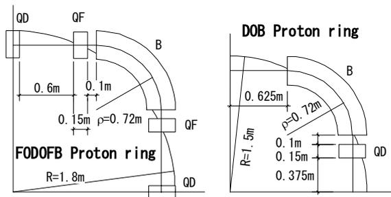
Figure 1: Layouts of the compact proton synchrotron (FODOFB and DOB versions).
