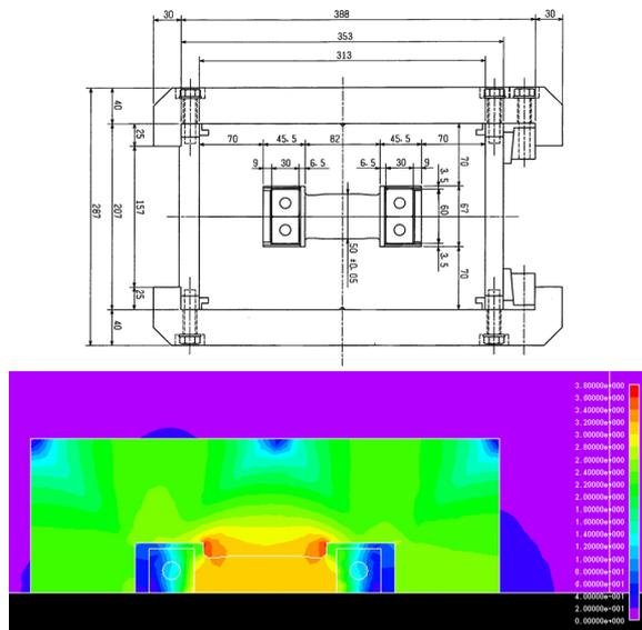
Figure 2: Cross-sectional dimensions of the dipole (top), and field distribution at max. excitation (bottom).
