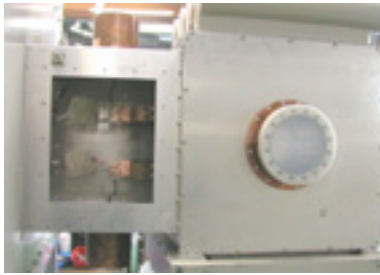
Figure 8: Developed broadband high voltage probes for rf cavity.
