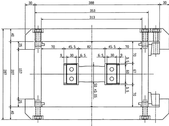
Figure 2: Cross-sectional dimensions of the dipole.
