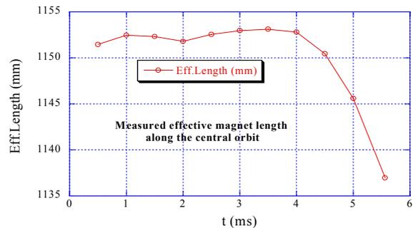
Figure 7: Measured effective magnet length.
