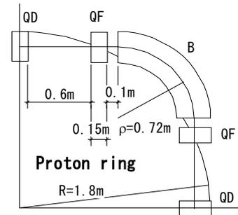
Figure 1: Layout of the compact proton synchrotron.
