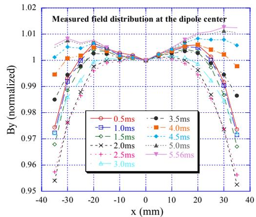
Figure 6: Measured field distributions.
