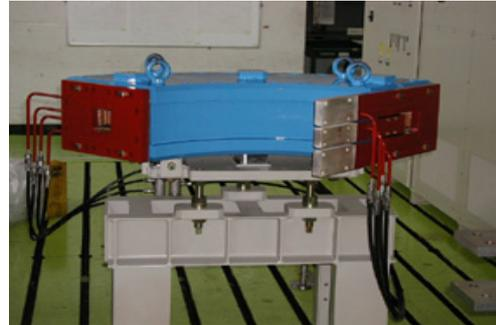
Figure 5: Completed dipole magnet.
