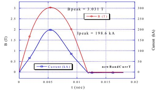
Figure 10: Measured time-dependent excitation curve.
