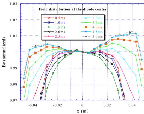
Figure 3: Field distribution at the dipole center without correction windings at every 0.5 msec.
