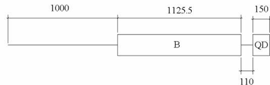
Figure 1: Superperiod of the proton synchrotron lattice for the missing QF version (unit: mm).
