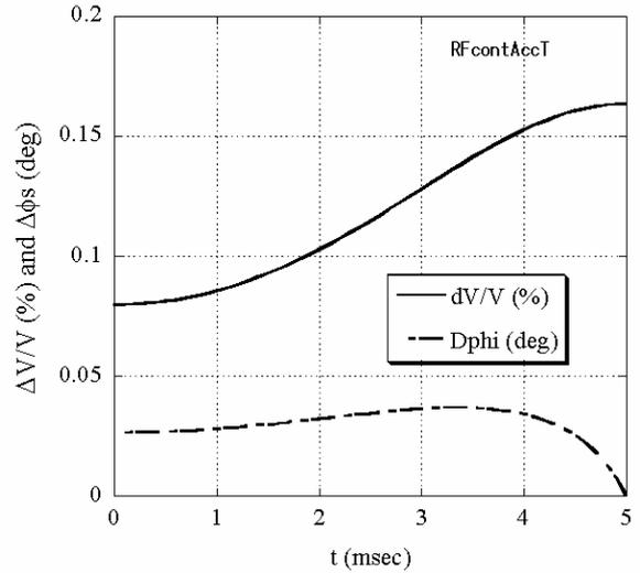
Figure 13: Accuracy of the gap voltage and phase control.
