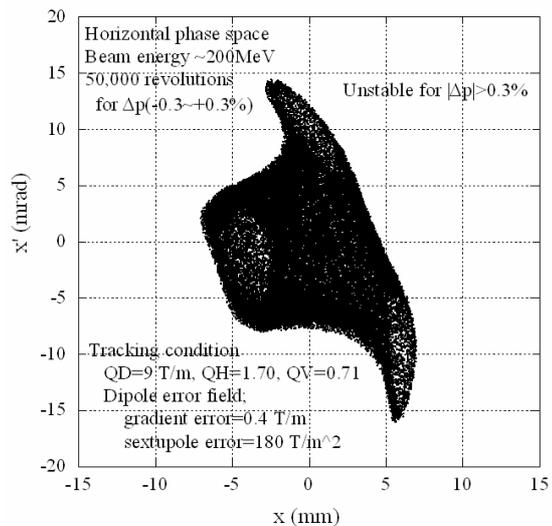
Figure 9: Sextupole error field of the dipole magnet is corrected with 4 sextupole magnets for proton with momentum of  $-0.3\% < \Delta p < 0.3\%$  at 200 MeV.
