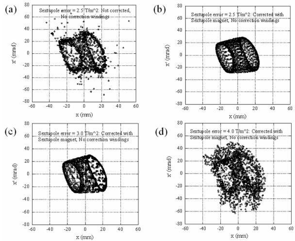
Figure 7: Proton behavior in the error sextupole field of the dipole magnet, (a) not corrected for 2.5 T/m<sup>2</sup>, (b-d) corrected for 2.5, 3.0 and 4.0 T/m<sup>2</sup>, respectively.
