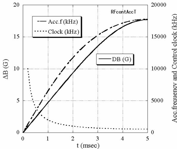
Figure 12: Control clock rate to attain the frequency error of 0.05%.  $\Delta B$  corresponds to the 0.05% frequency step at each time.
