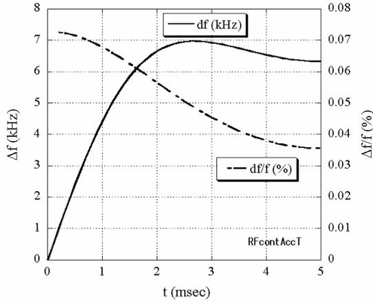
Figure 11: Accuracy of the acceleration frequency to attain the orbit error less than 1 mm in the dipole magnet.
