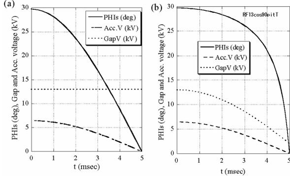
Figure 10: Required RF phase for the gap voltage: (a) 13 kV constant, (b) reduced according to  $13\cos(90\pi t)$  kV.
