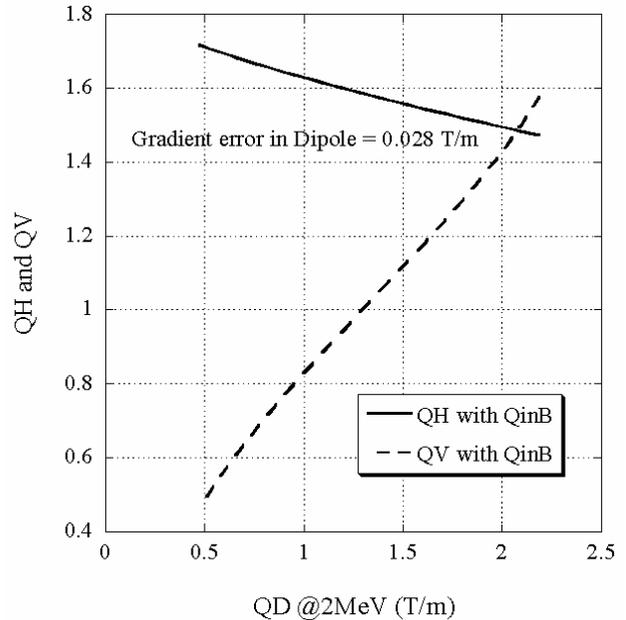
Figure 5: Tune variation by the field gradient of QD at injection when the gradient error of Fig.4 is considered.
