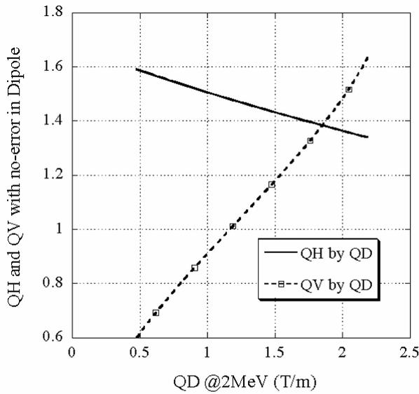
Figure 3: Tune variation by the defocusing quadrupole magnet QD at injection (2 MeV).
