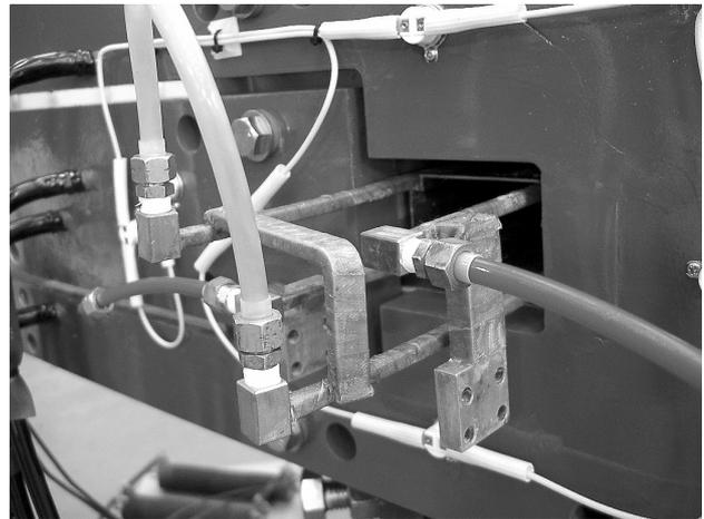
Figure 8: Correction coil in the dipole magnet gap.
