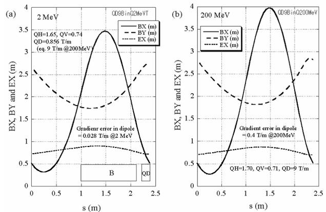
Figure 2: Beam parameters for the missing QF version. (a) QD=0.856 T/m at 2 MeV, (b) QD=9 T/m at 200 MeV.
