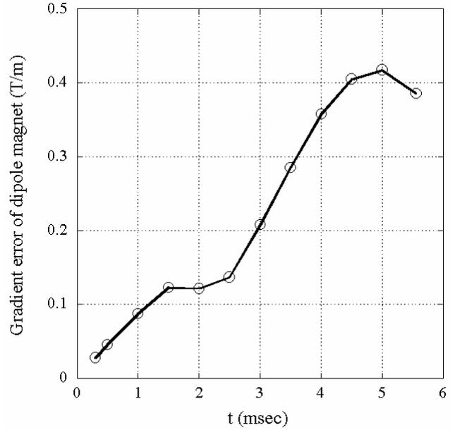
Figure 4: Measured gradient error averaged over the whole length of the dipole magnet.
