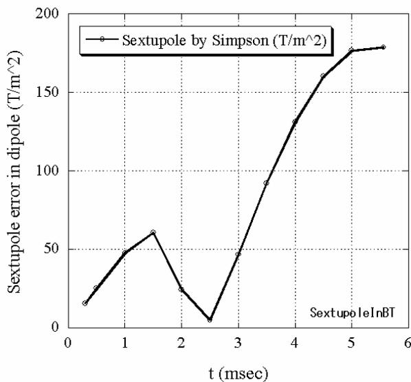
Figure 6: Sextupole field component in the dipole magnet.
