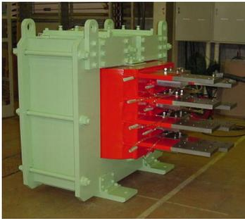
Figure 13: Step-down transformer.
