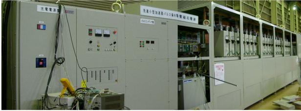
Figure 12: Pulsed power supply equipped with an additional capacitor. Two separate pictures are merged at the middle.
